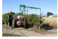
Fig. 1. Over the row boom application of mycoinsecticides to red raspberry hills.
