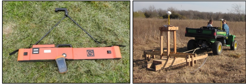
Figure 1. The Geonics EM38-MK2 (left) and an example of a utility vehicle pulling the EM38 in a sled for non-invasive soil mapping (right).
