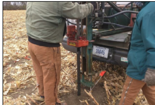
Figure 3. Truck-mounted penetrometer similar to the one to be used in this proposed study.
