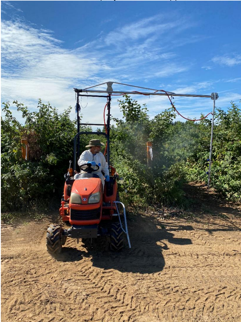
Photo 1. Over-the-row sprayer used for applications.
